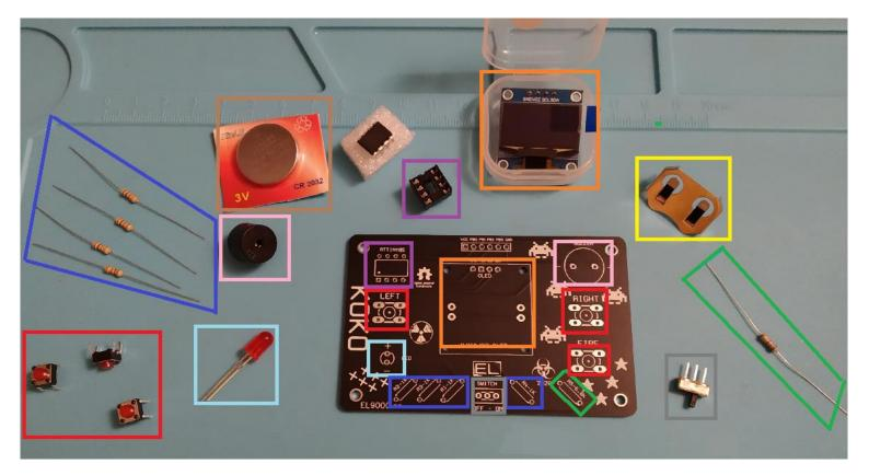
The 6 pin header, on the top of the pcb, is not in the picture but it's included. It's very important the position of the positive/negative pole for <u>LED</u> and <u>Buzzer</u>. Carefully look below at the position of the <u>battery holder</u> on the back of the pcb, otherwise you will not be able to insert the battery!
